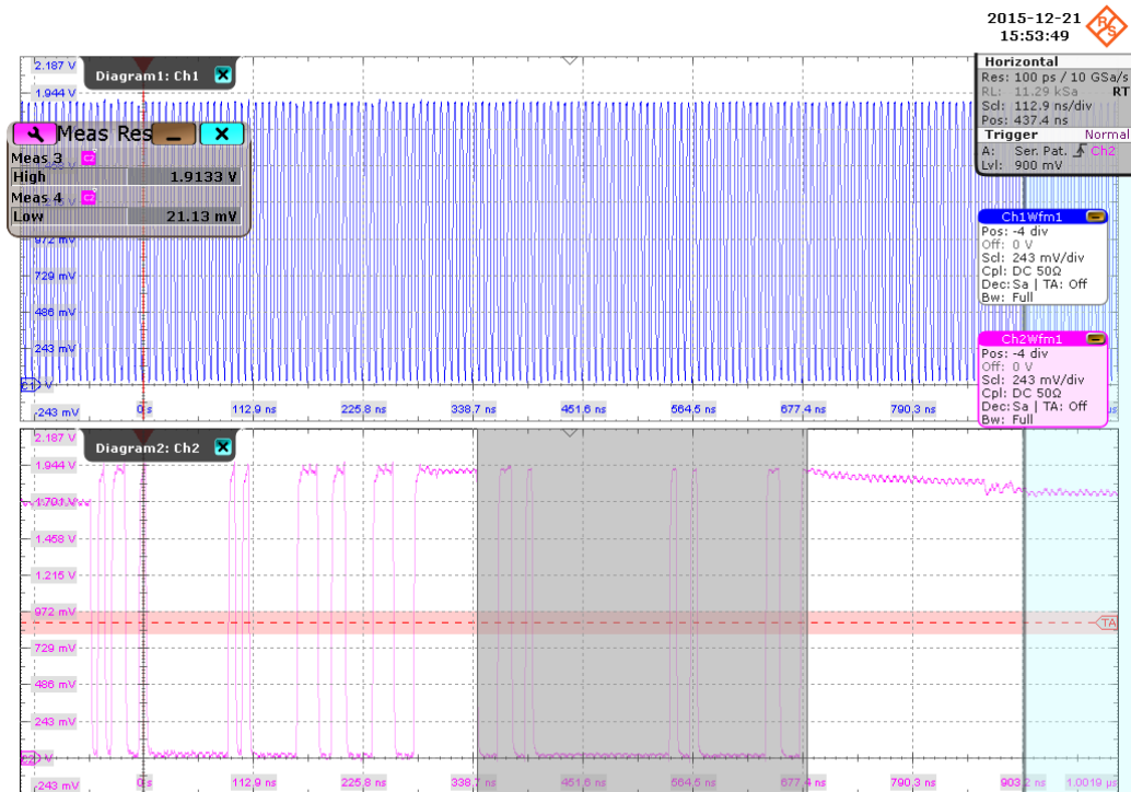
Figure 4-5: HS200 CMD Push Pull output level voltage
